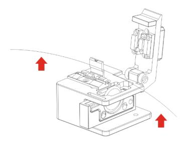
Open fixing plate and cover, take fiber out, don't touch the terminal of fiber, so as not to damage the fiber. please clean the rubbish or dirt on blade in time, so as not to damage the blade.
