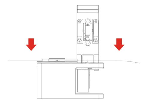
Fine tune the screws on the blade base and lift the top of blade base to the fiber.
