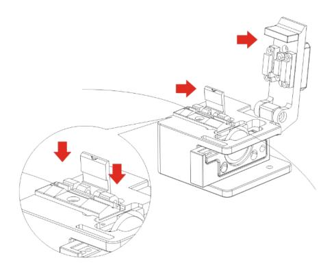
Open cover and fixing plate, place one piece of fiber (which was stripped coating and cleaned ) on the V-groove.
