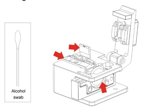
After one period time of use please clean groove, fixing plate and blade edge by alcohol(don't use acetone or other corrosive solvent).
