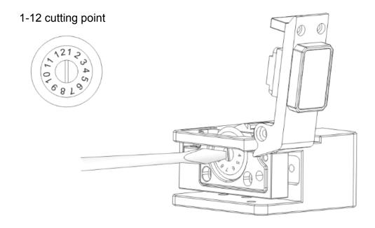
Use screw drive anticlockwise drive the screw , anticlockwise rotate the blade to next cutting point, then tighten the screw .
