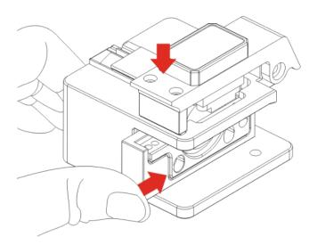
Close fixing plate and cover, push slider to the end.
